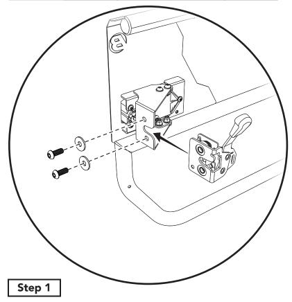
Attach the Rotor Assemblies to the Rotor Brackets.
